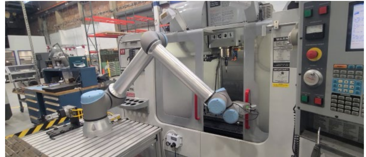
Pilot run of 2,550 clamps made with robotic machine tending
