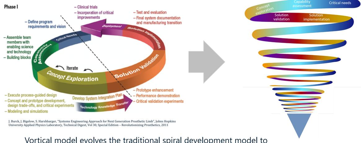
Vortical model evolves the traditional spiral development model to reflect the tightening of corresponding spirals as the model refinement/ progression continues.
