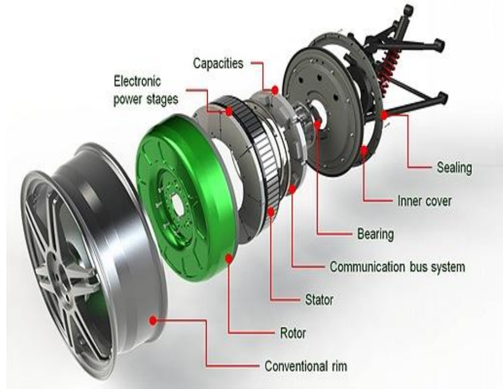
Exploded View of Protean Motor
